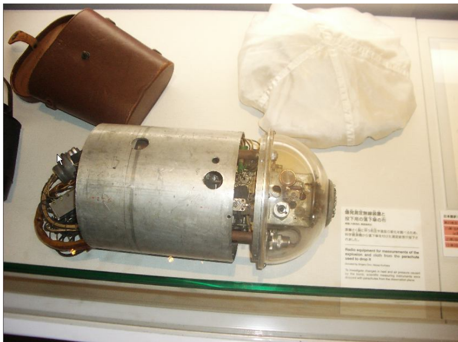
Radio equipment for measurements of the explosion and cloth from the parachute used to drop it. Hiroshima Peace Museum. (Photo courtesy of Ben Rusek, NAS CISAC)
